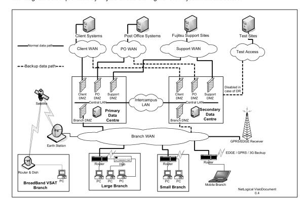
The diagram below provided by Fujitsu shows the high level IT system infrastructure:
